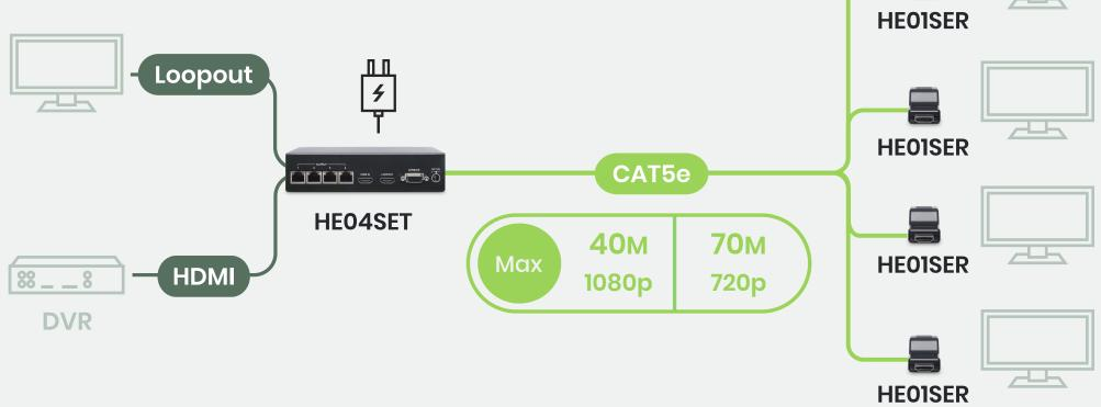
better) cables to extend a 1080p HDMI signal for up to 40M.
